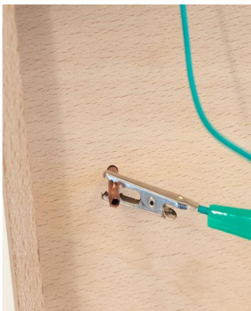
Figure 11: crocodile clip can be attached at the bottom to the copper tube inserted through.
