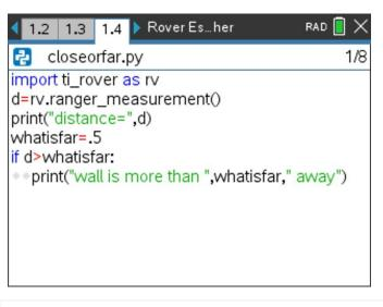
Task: Use the Rover ranger to detect distance to an object, print the distance.
